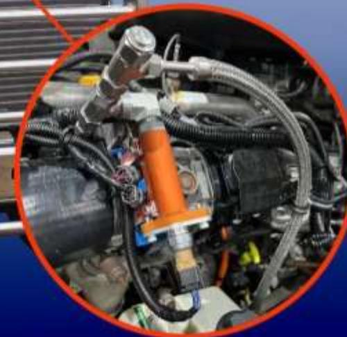
H2 injection manifold in-line with air intake
